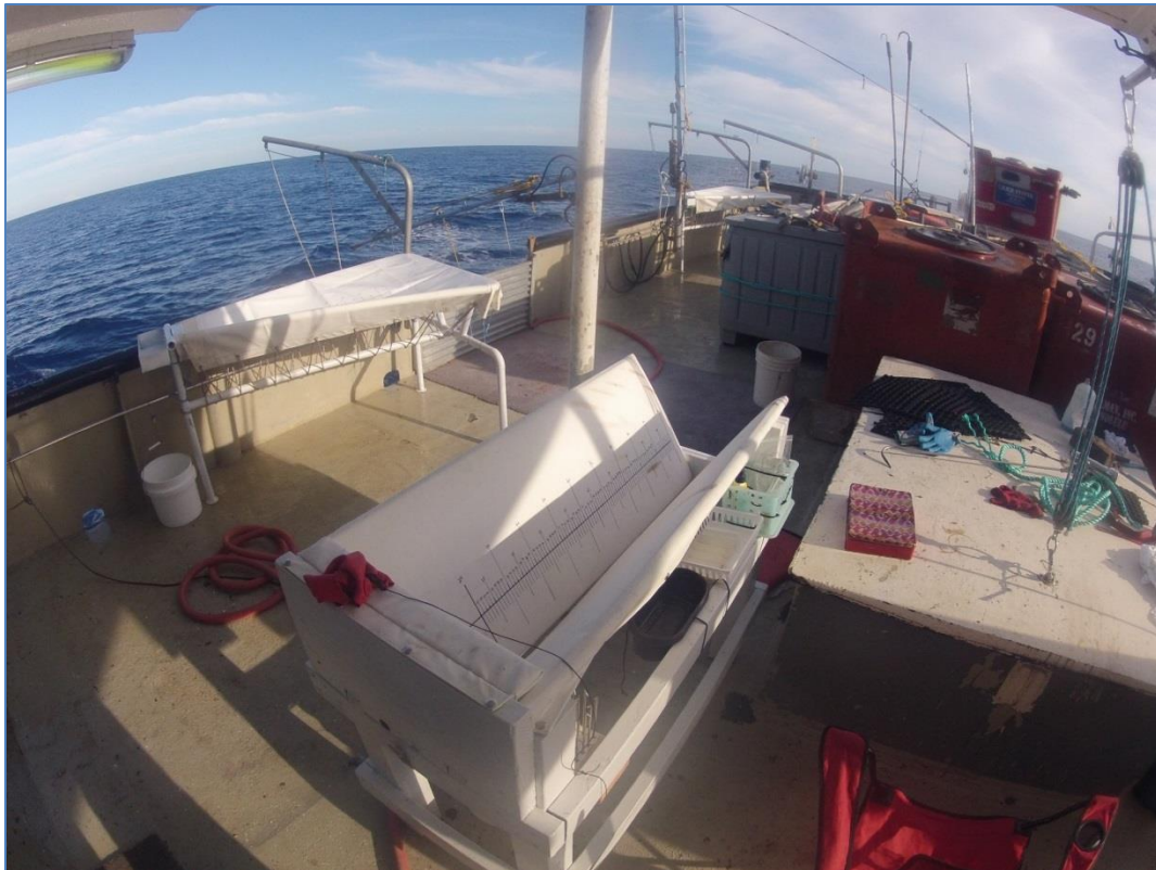
Picture 2: Archival tagging cradle (first plan) and 2 starboard side conventional cradles. Part of the dangler gear and the stern hydraulic reels can also be seen in the picture.
