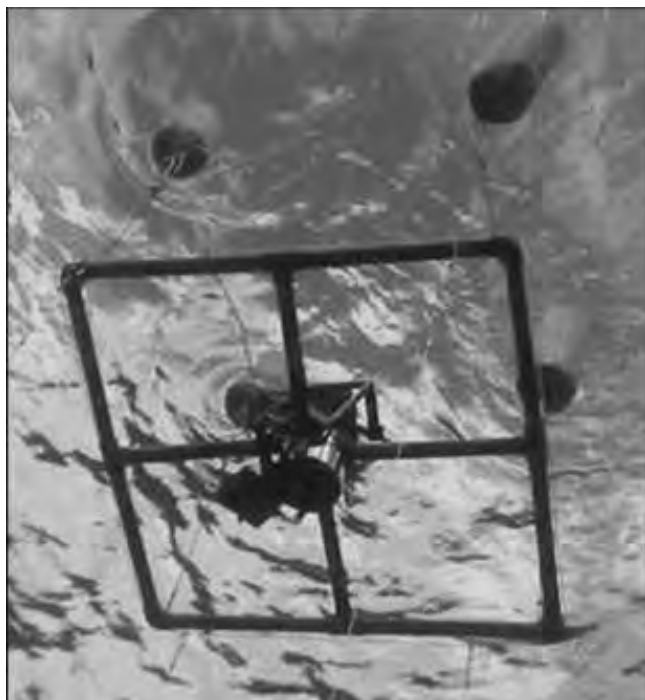
Figure 2 - The support was maintained at the sea surface by four buoys, and equipped with four branchlines at each corner, and a camcorder at its centre (interaction tests with platforms)
