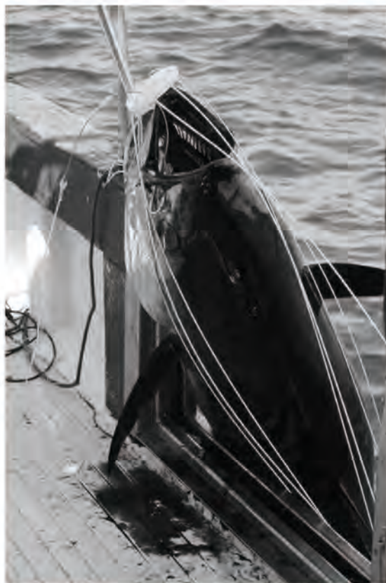
Fig. 1. A baited tuna covered by spider. The spider is a device made up of eight polyester legs. The legs are maintained by using a 100 mm diameter plastic disc, with 16 holes in its outer range and a 37 mm diameter central hole through which the hooked branchline is inserted. The triggering system consists of a beta pin through which the line was inserted and was tightened by an elastic ring. The whole system could only be released by a pulling of the hooked fish on the branchline.
