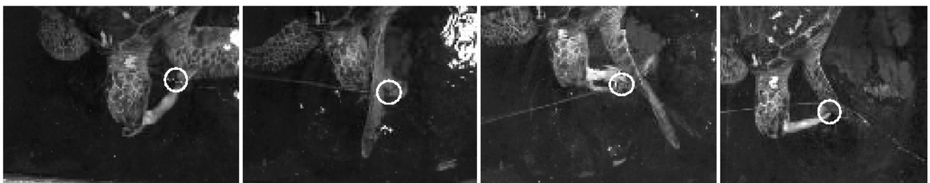
Fig 2. Single frame capture series of a green turtle using its front flipper to help remove squid bait from the Smart Hook (white circles indicate position of the Smart Hook ). Despite frequent use of the forelimb the guard very successfully prevents foul-hooking in the flipper.
