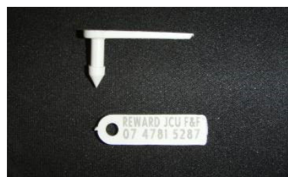
Fig 2: Rototag male (top) and female (bottom) sections. (Source: Michelle Heupel)
