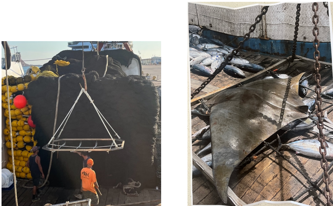
Figure 1. Sorting grid (left) and a Manta released using the sorting grid (right)
