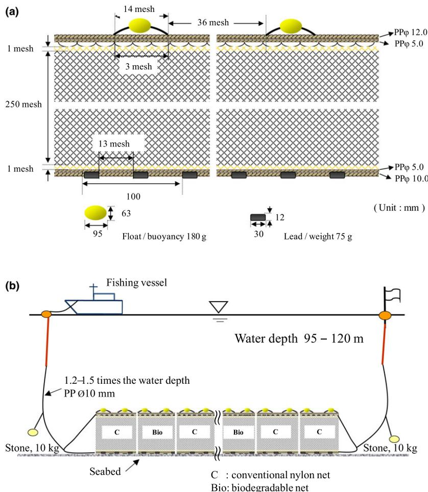
**Figure 2** A schematic presentation of (a) the construction of the experimental driftnet for yellow croaker and (b) the layout of netting panels in the experimental fishing.
