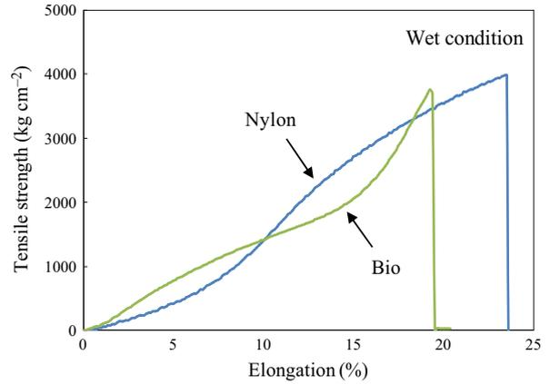
**Figure 4** Pooled strength and elongation curves of knotless monofilament. Dry indicates that the specimens were dry and had not been immersed in water. Wet indicates that the specimens were wet after having been immersed in distilled water for 24 h. ‘Nylon’ signifies nylon monofilament, ‘bio’ signifies biodegradable monofilament.
