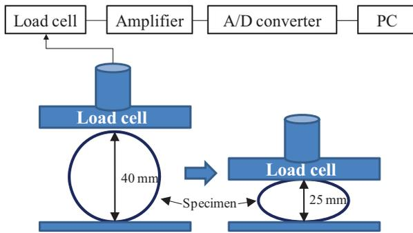
**Figure 1** A schematic concept for measuring the stiffness of the monofilaments by Brandt's method.
