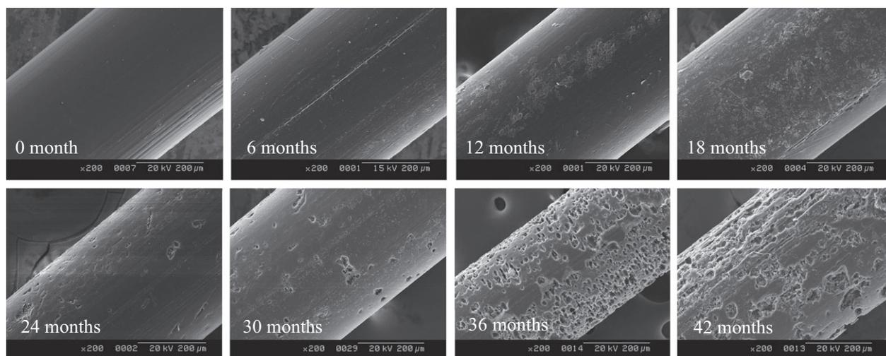
**Figure 7** The degradation process of the immersed biodegradable monofilament observed with a scanning electron microscope. Pictures show the degradation states at 6-month intervals up to 42 months.
