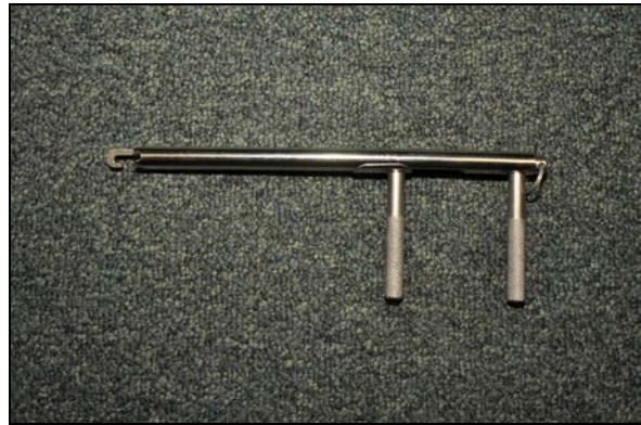
Figure 35. Squeeze handle dehooker (e.g., Fish Hook Extractor ® ) (NMFS/SEFSC photo).
