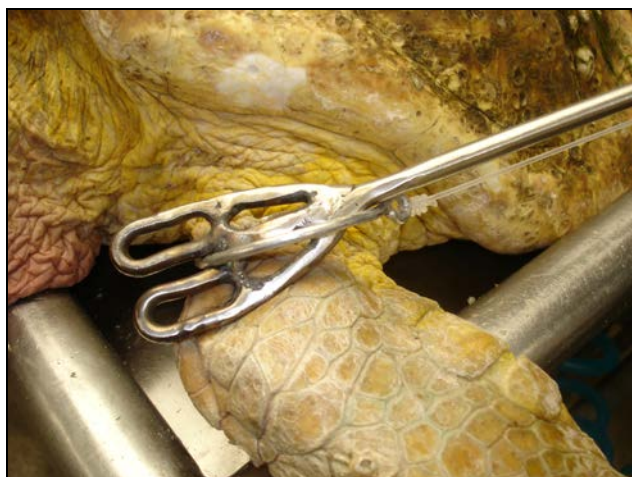
Figure 31. Chain-link dehooker (NMFS/SEFSC photo).
