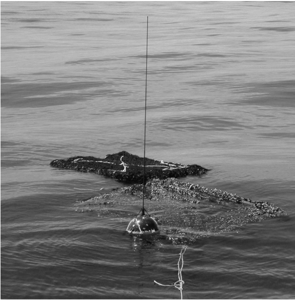
Fig. 1. A typical FAD constructed from a bamboo raft with netting hung beneath and a buoy fitted with location-tracking technology. Photo copyright: FADIO/IRD-Ilfremer/B. Wendling.
