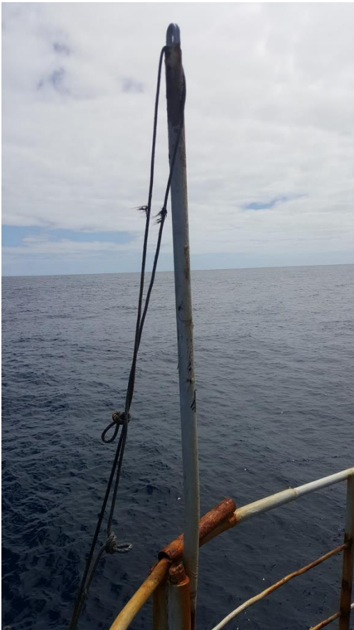
Figure 3. Image from a transshipment observer of a tuna longliner showing a tori pole that was not considered structurally sound. It lacks back stays or other strengthening systems
