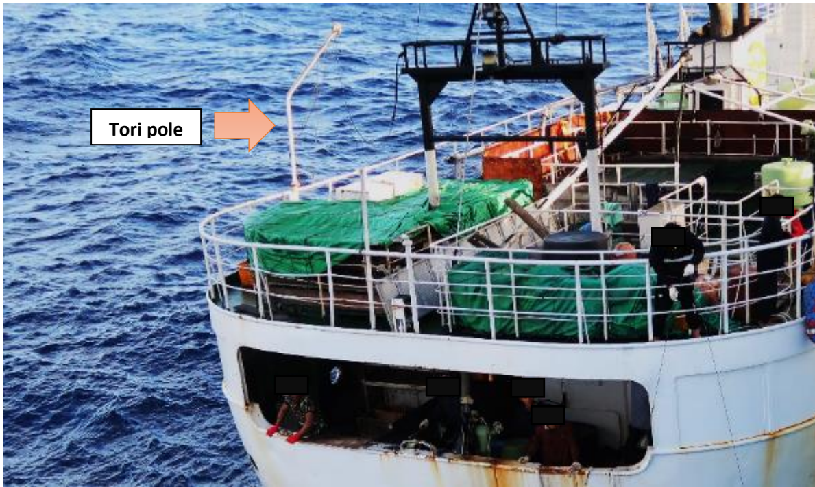
Figure A9. An alternative design for a best practice tori pole.
