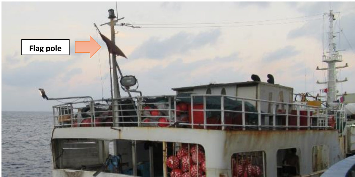
Figure A3. Note the flag pole, which is not a tori pole or BSL attachment point.
