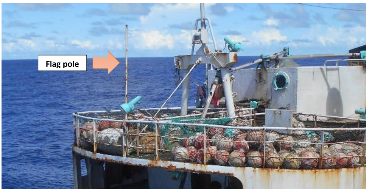
Figure A7. Flag pole attachment point. These are not torii poles and would not be able to withstand the drag of a BSL. During PBO visits, some captains have tried to sell this as a BSL mounting position.
