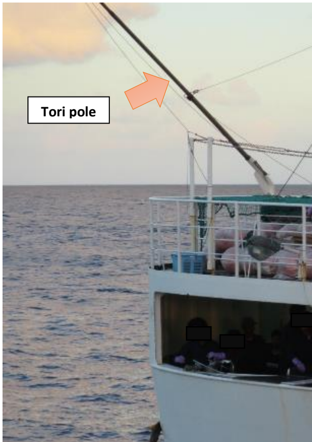
Figure A5. A good example of a torii pole mounted over the bait casting area. Even though the photo only includes part of the TP, it is clearly higher than 7m above the waterline and would qualify as a best practice (BP) installation.
