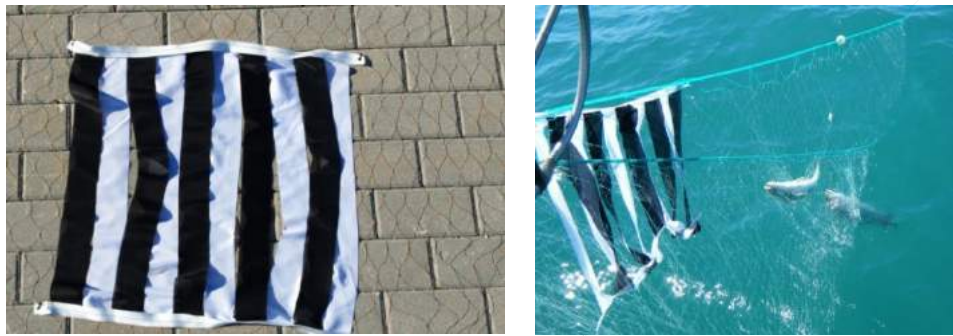
Figure 15. Drag-reducing contrast net panel in a grating pattern ( left ) attached to the fishing net ( right ). (Images: Julius Morkunas, Seabird Task Force, from Crawford et al. (2016) and SPEA from seabirdbycatch.com)
