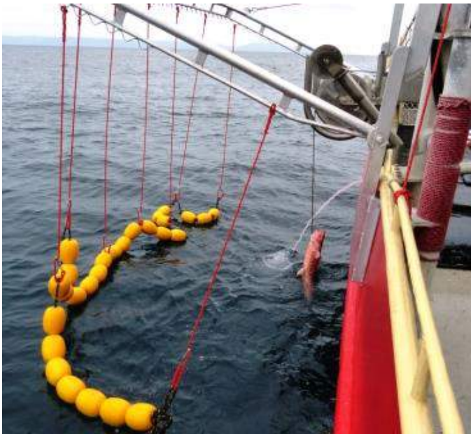
Figure 7. Brickle curtain. (Image: Australian Fisheries Management Authority)
