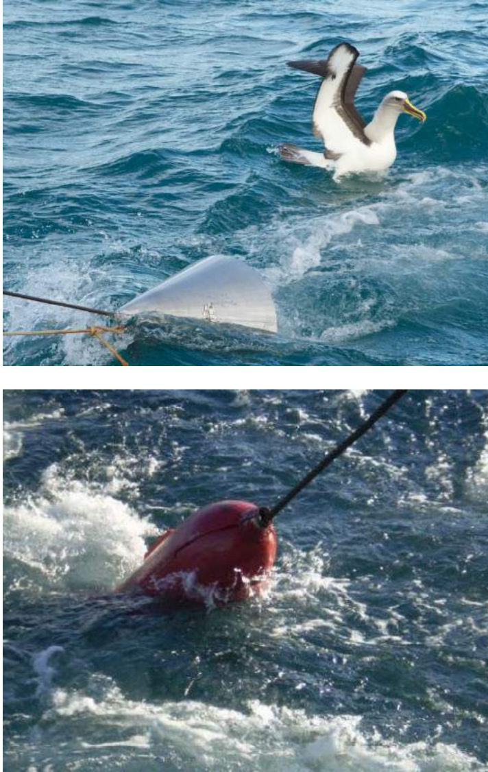
Figure 13. Top: Cone deployed on in-shore trawl warp cable to prevent seabird strike on the warp cables at the warp-water interface (Image: J. Molloy). Bottom: The Seabird Control Unit Device (SCUD) (Guild 2007)
