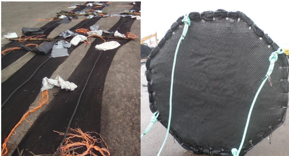
Figure 2. Example of non-entangling FADs constructed in Abidjan and used in the Atlantic Ocean
