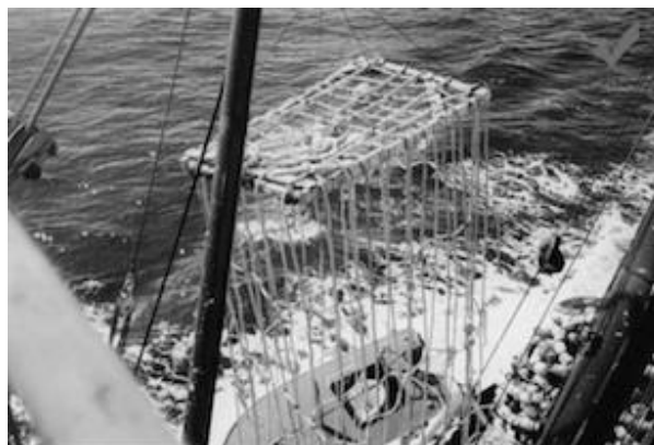
Fig 6. Device with uncovered raft and submersed part made of loose ropes
