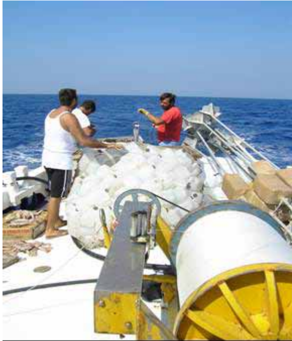
Figure 17 Setting procedure of the longline using the winch
