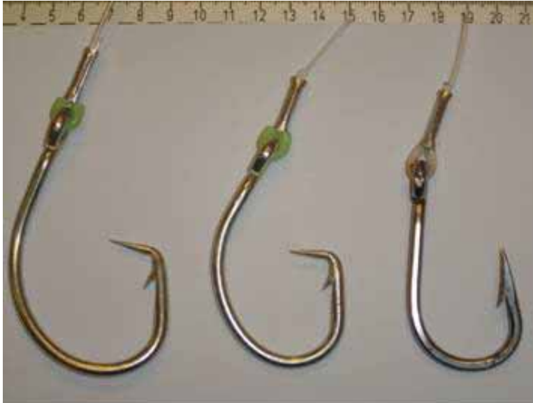
Figure 14 The three hook types used in the Eastern Mediterranean trials (circle 18/0, circle 16/0, J)
