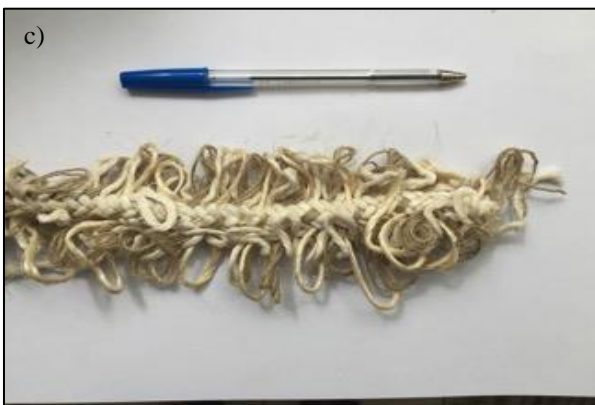
Figure 1. Biodegradable ropes selected for the tests (a) 100 % Cotton rope b) 50% cotton and 50% sisal rope c) Cotton, sisal and linen rope with loops.
