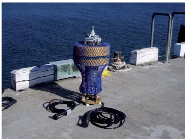
A prototype GDS buoy with two hydrophones.
