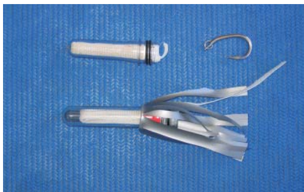
Two variations of polycarbonate streamer containers holding wire-embedded electric fence tape. The typical hook-to-tube distance was 50 cm.
