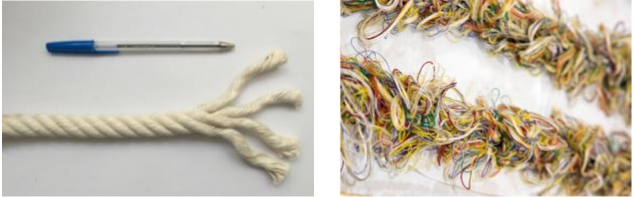
Figure 4. Left: 20 mm cotton rope; Right: Cotton rope with loops to allow bio-fouling.
