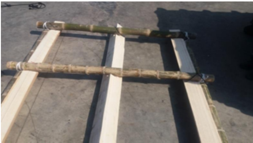
Figure 7. First prototypes deployed at sea using as floats balsa wood and bamboo canes
