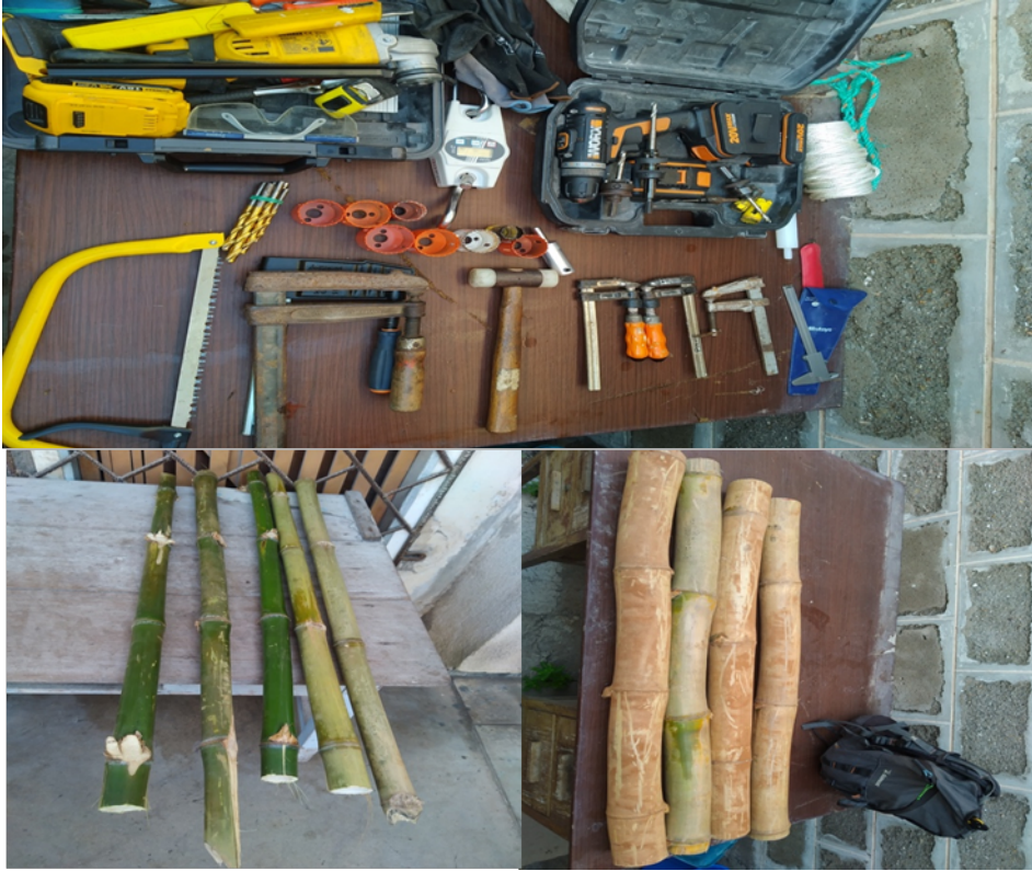
Figure 45. Tools and bamboo canes needed to build the biodegradable FAD.
