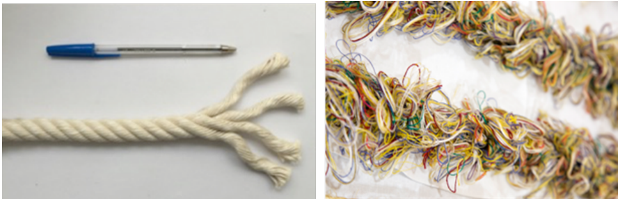
Figure 15. Left: 20 mm cotton rope; Right: Cotton rope with loops to allow bio-fouling
