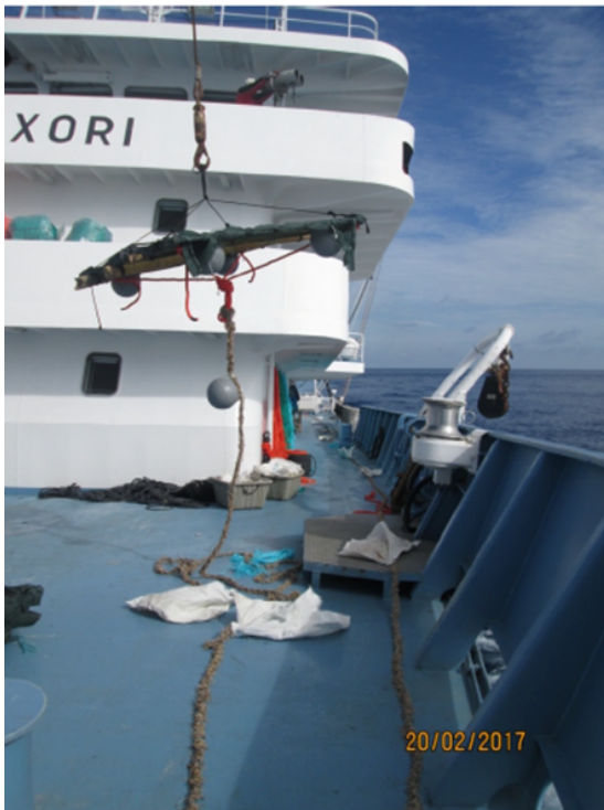
Figure 29. FAD type 2: A single rope hanging from the center of the rope. This design was used at 30m, 50m and 70m depth.
