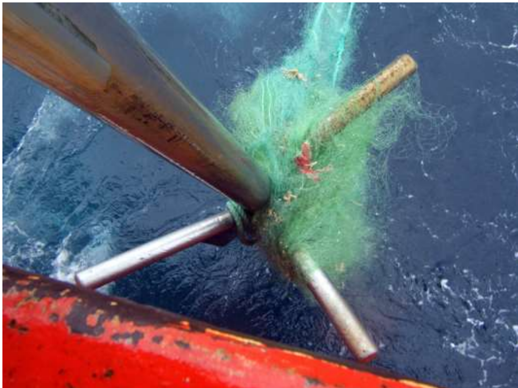
Figure 2.4: Recovering ALDFG using a “creeper” (Large et al. 2006, © Crown Copyright)
