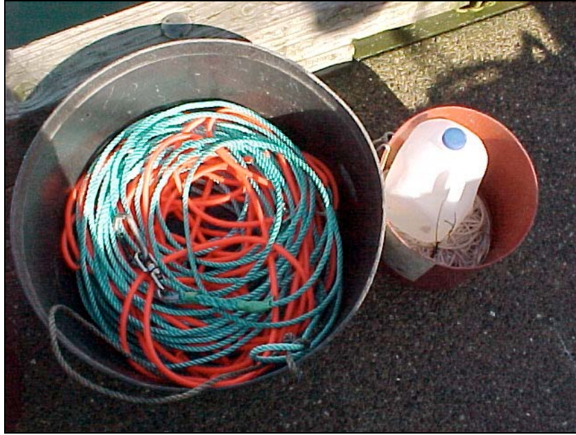
Figure 13: USFWS streamer line (left) and Hull line and jug (right).
