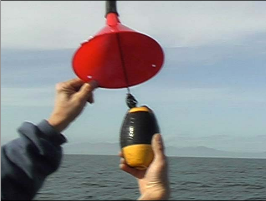
Figure 3: Funnel and buoy used to create drag on streamer line.
