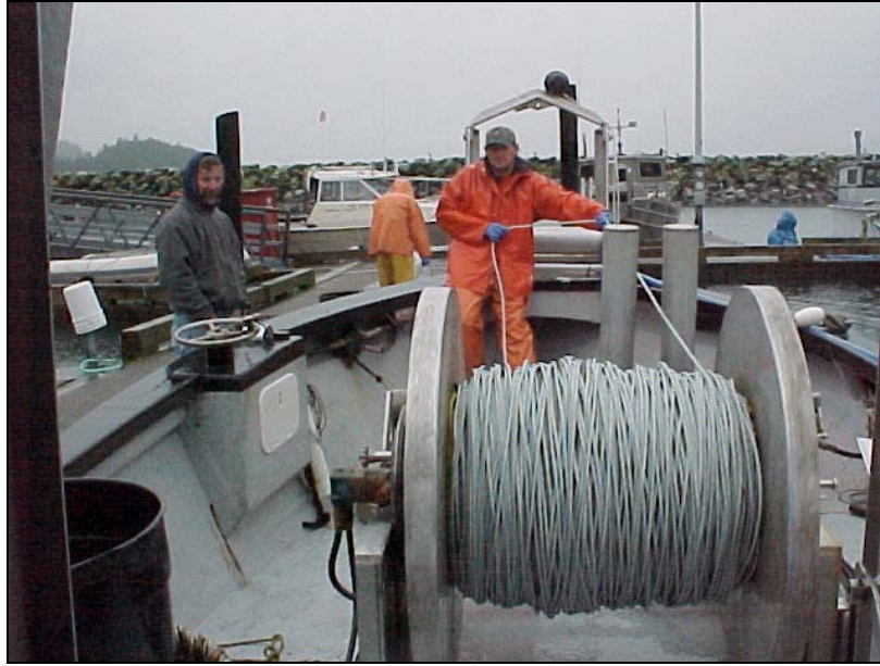
Figure 6: Adding test gear to hydraulic reel. F/V Salmo
