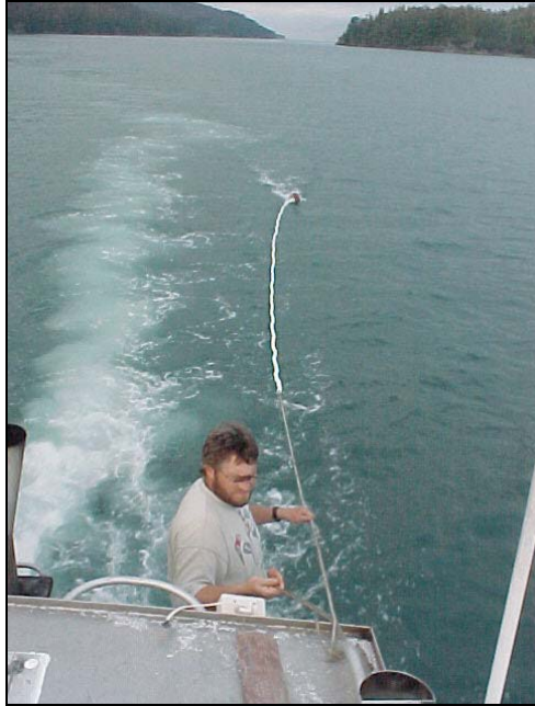
Figure 11: Deploying Rule hose buoy line. F/V Cape Fear
