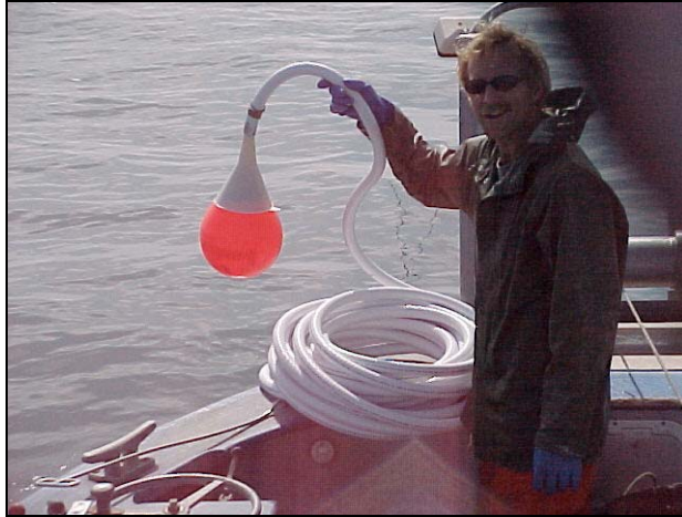
Figure 7: 1" Trident hose, number "0" buoy, and plastic funnel knot protector. F/V Jitterbug
