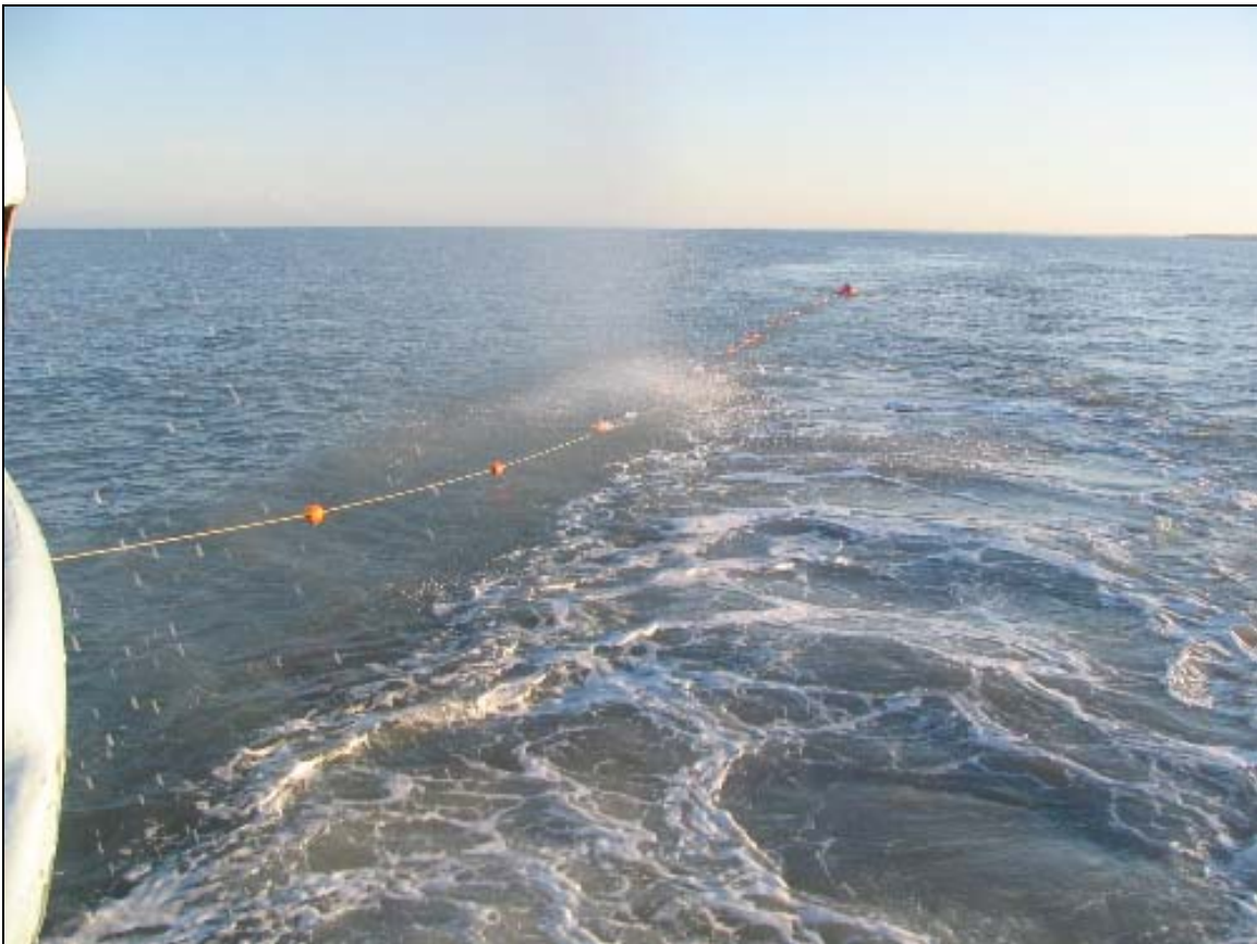
Figure 15: Water spray hitting measuring line marked at 5 m intervals.
