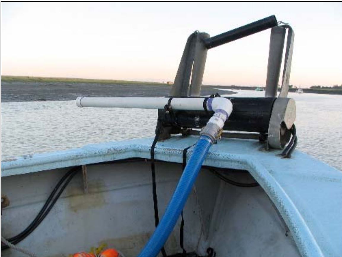
Figure 14: The water-spray device developed by Heidemann.
