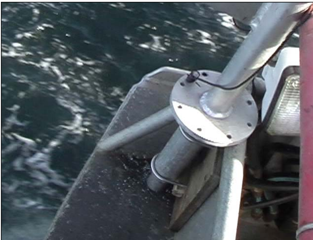
Figure 2: Davit swivel mechanism.
