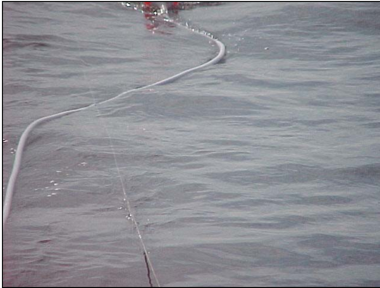
Figure 10: One inch Trident hose buoy line crossing over groundline. F/V Jitterbug
