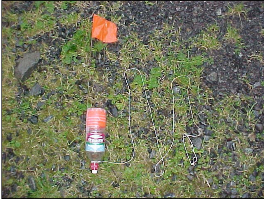
Figure 4: Plastic water bottle, flagging, and 2-m line with snap.
