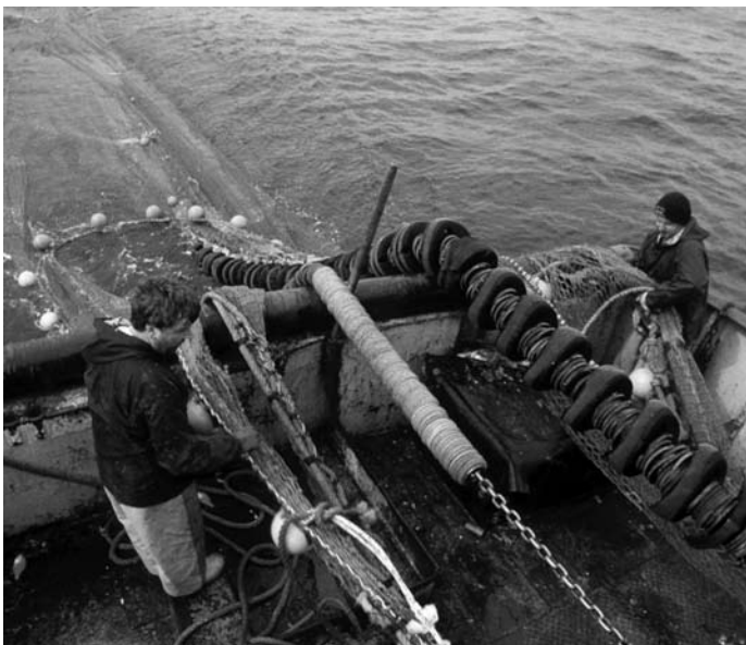
Shooting away the trawl on a North Sea trawler. © WWF-Canon / Quentin Bates
