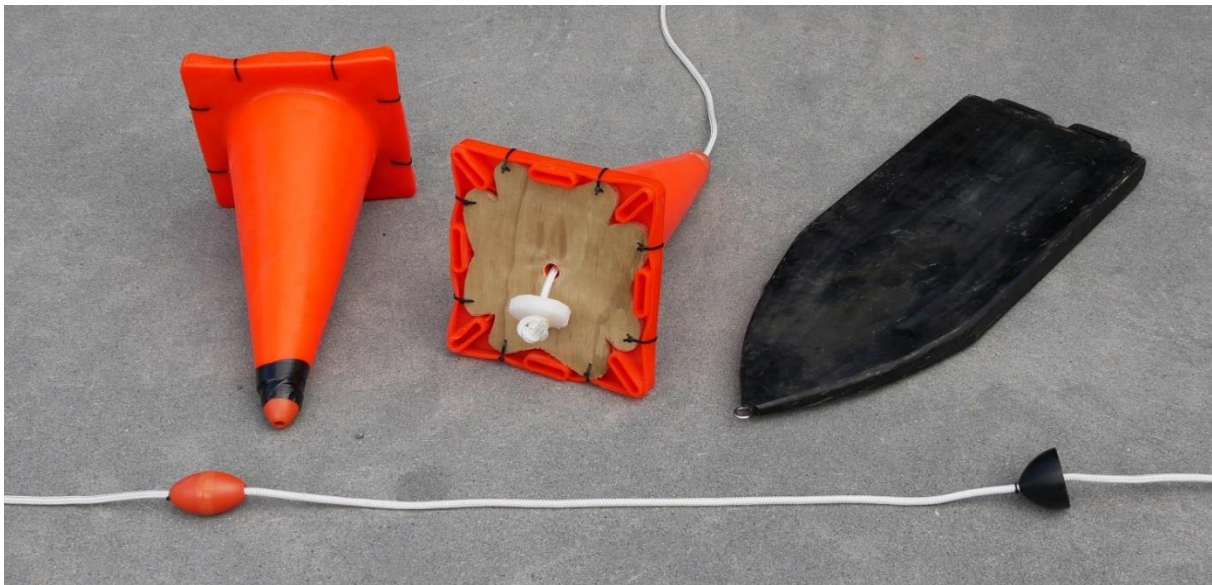
Figure 4: Drag section components for demersal longliners.
