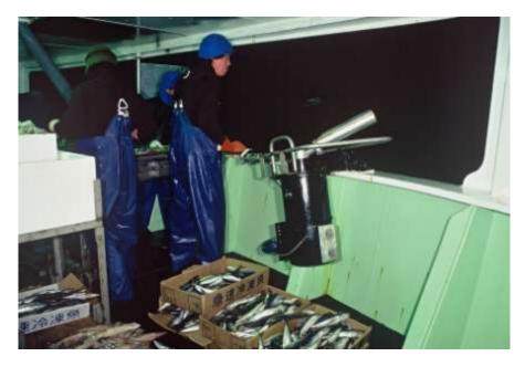
Figure 2. Japanese-made "Tuna Mate" bait casting machine in operation on a Japanese tuna vessel fishing out of Hobart (under the CCSBT agreement) in the mid 1990's. Still photography does not impart an accurate impression of the velocity of the cast which, in this case, straightened the 40 m branch line. Baited hooks landed in clear (un-aerated) water 15-20 m outboard of the streaming position of the bird scaring streamer line.
