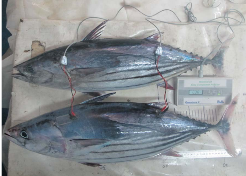
Figure 8. BIA electrodes inserted to large, unassociated skipjack (photo F. Forget)
