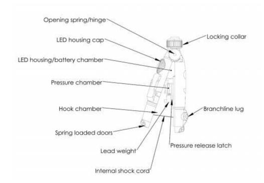
Figure 1. Components of the Hook Pod
