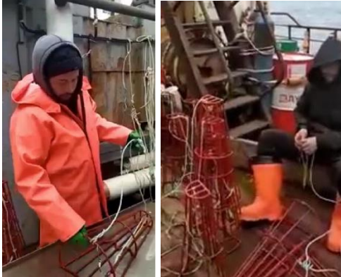
Figure 7. Steel protection frame being used in a Russian fishery (from A. Stubbs presentation).
