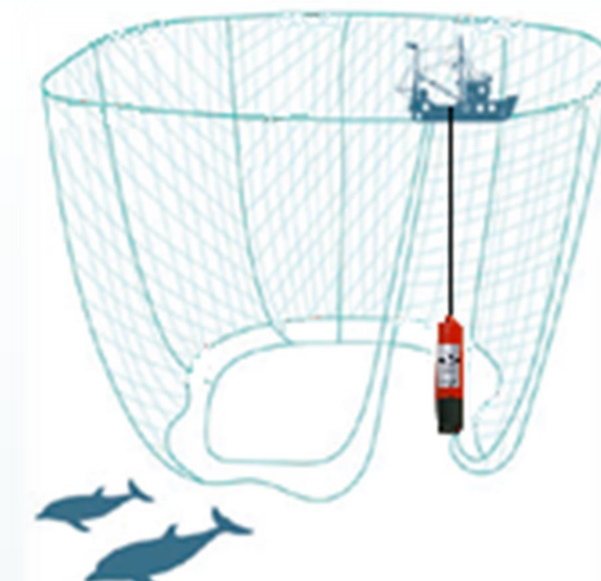
Fig. 6: Assembly of the pinger on a purse seine vessel.
