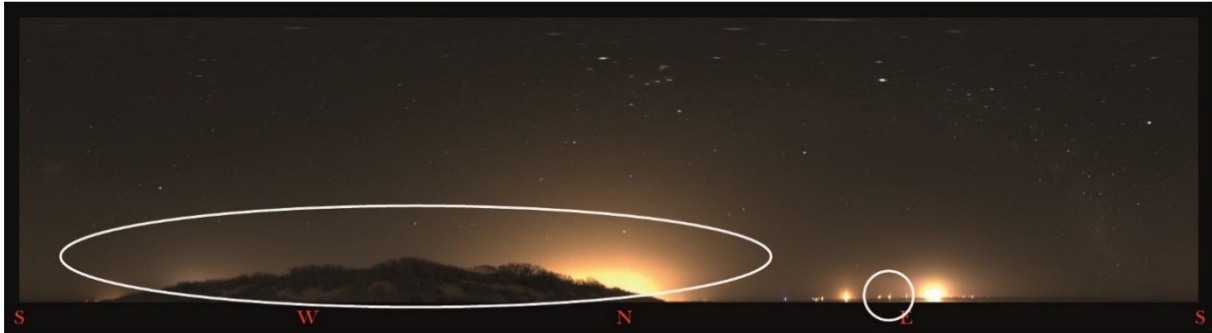
Circled left: lights shielded by vegetation screen. Circled right: point sources of light directly visible
