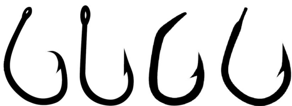
Fig. 1 Four hook designs commonly used in pelagic longline fisheries, from left, circle, J, tuna and teracima hooks. (Beverly 2009; IATTC 2011)
