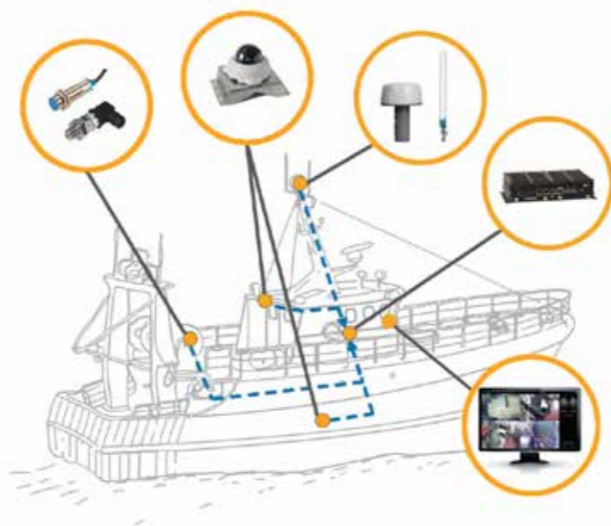
Figure 1. Generalised layout of a REM system, showing (from left to right) gear activity sensors, camera (digital or analogue), GPS and communications antennae, central control box with integrated storage and a GUI (graphical user interface) display screen (courtesy of Anchorlab).
