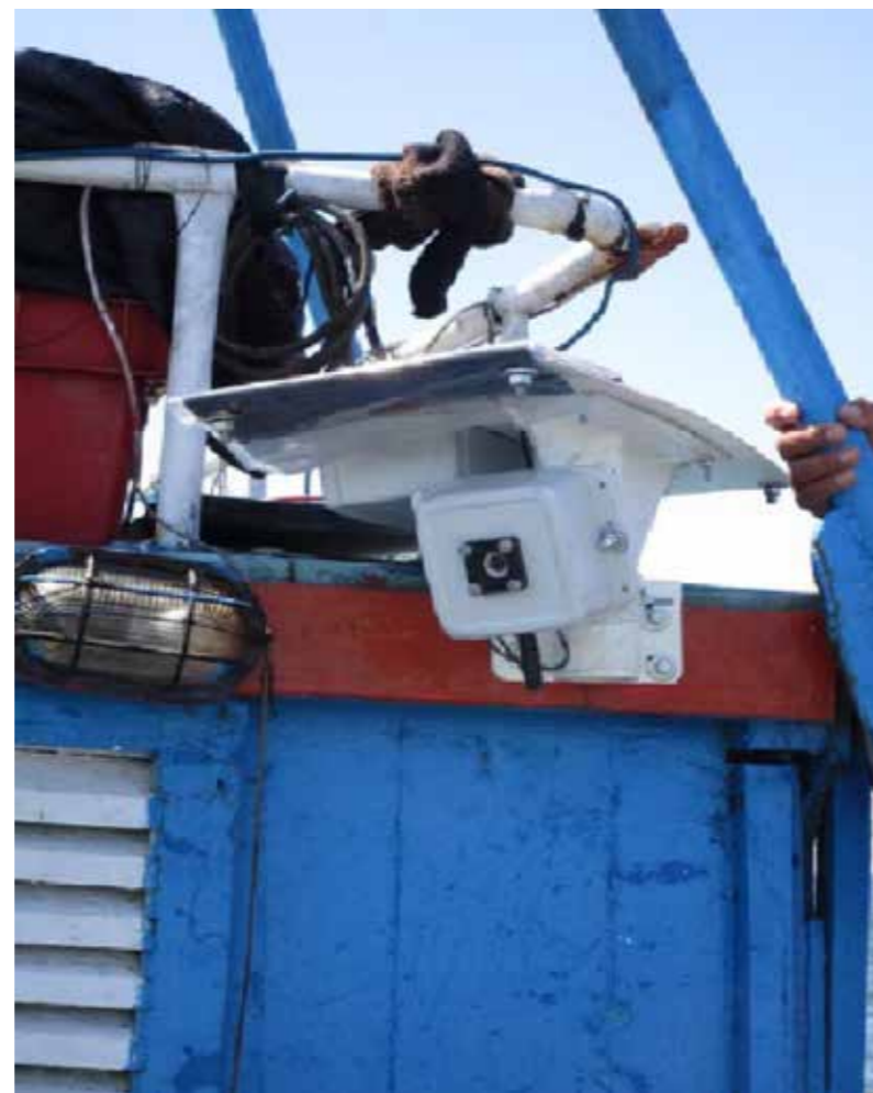
Figure 20. The Shellcatch REM system for monitoring small scale fisheries [92].
