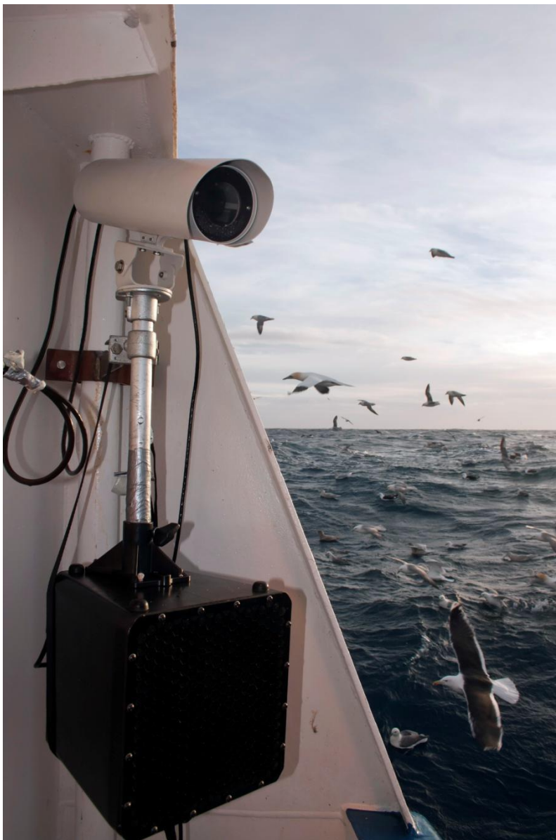
Figure 3: The Installed prototype set-up, with the laser on top and the sound system on the bottom.
