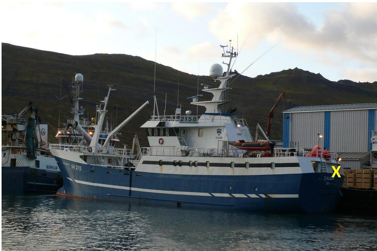
Figure 1: The longline vessel Tjaldur moored at the coastal town of Rif. The yellow x marks the preferred location of the Seabird Saver in this vessel. The lines are shot out of the back just below this point.
