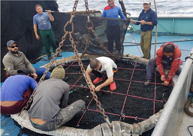
One version of a manta grid, designed by fishers, sits directly atop a "brailer" net so it can sort a mobulid out from other incoming catch. Crew can then use a winch to raise and release the mobulid. Image by TUNACONS/Cronin et al. 2022, *ICES Journal of Marine Science*.
